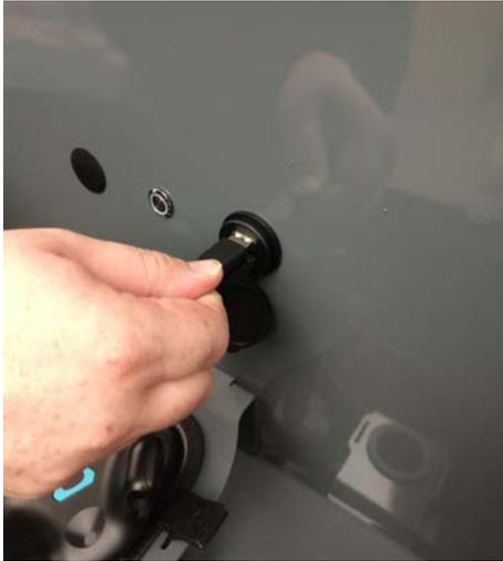
Clean up by disconnecting the keyboard and mouse from the unit, placing them back in the box on the back plate, securing the back plate, and screwing back in the two thumbscrews to the backplate.
